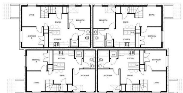
BASEMENT SUITE FLOOR PLAN 548 SQ. FT. / UNIT
